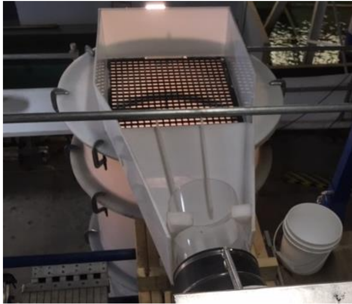
Figure 5 Test Loop Grated Inlet
