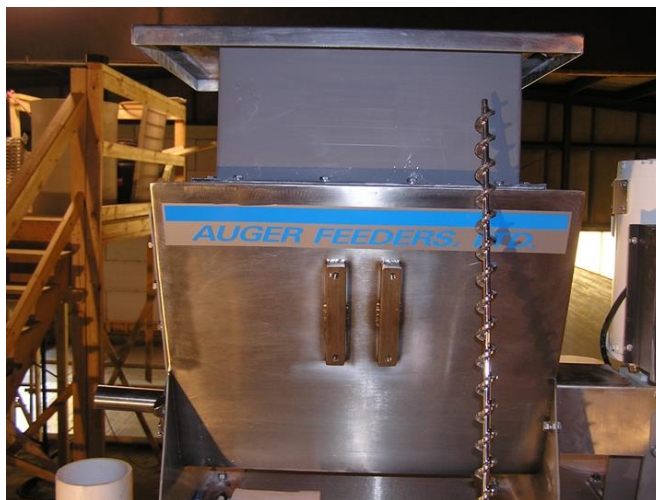
Figure 10 Photograph Showing Variable-Speed Auger Feeder
